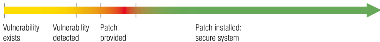
Fast installation of the patch reduces the time period marked in red, during which attacks are probable
